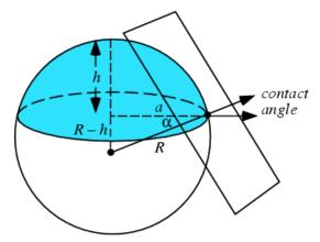
*Figure 1: Contact Angle Definition*
